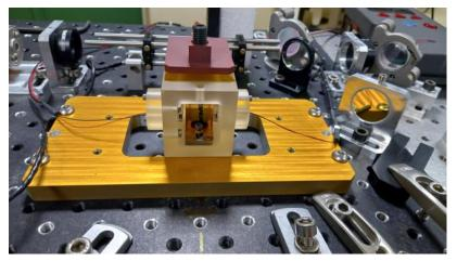
*Figure 2: Nested Cavity OPO zerodur cavity once aligned. The crystal is placed in the copper oven in the center, and the mirrors are aligned by translation on the zerodur body.*
