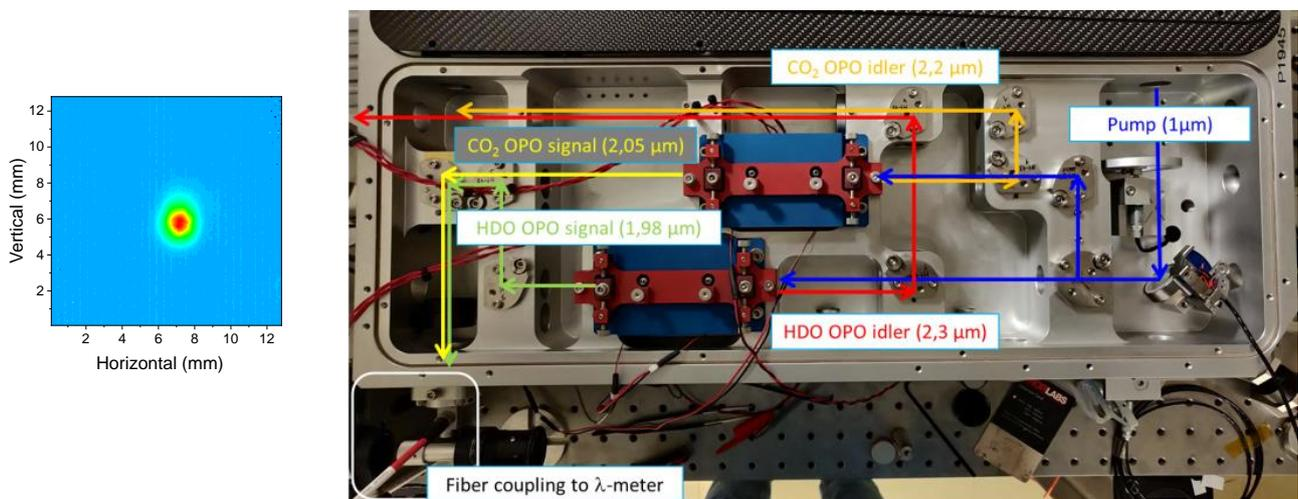
**Figure 3: First housing after integration of the two OPOs (Beam paths and wavelengths combinations are indicated) and OPO output beam (left).**
