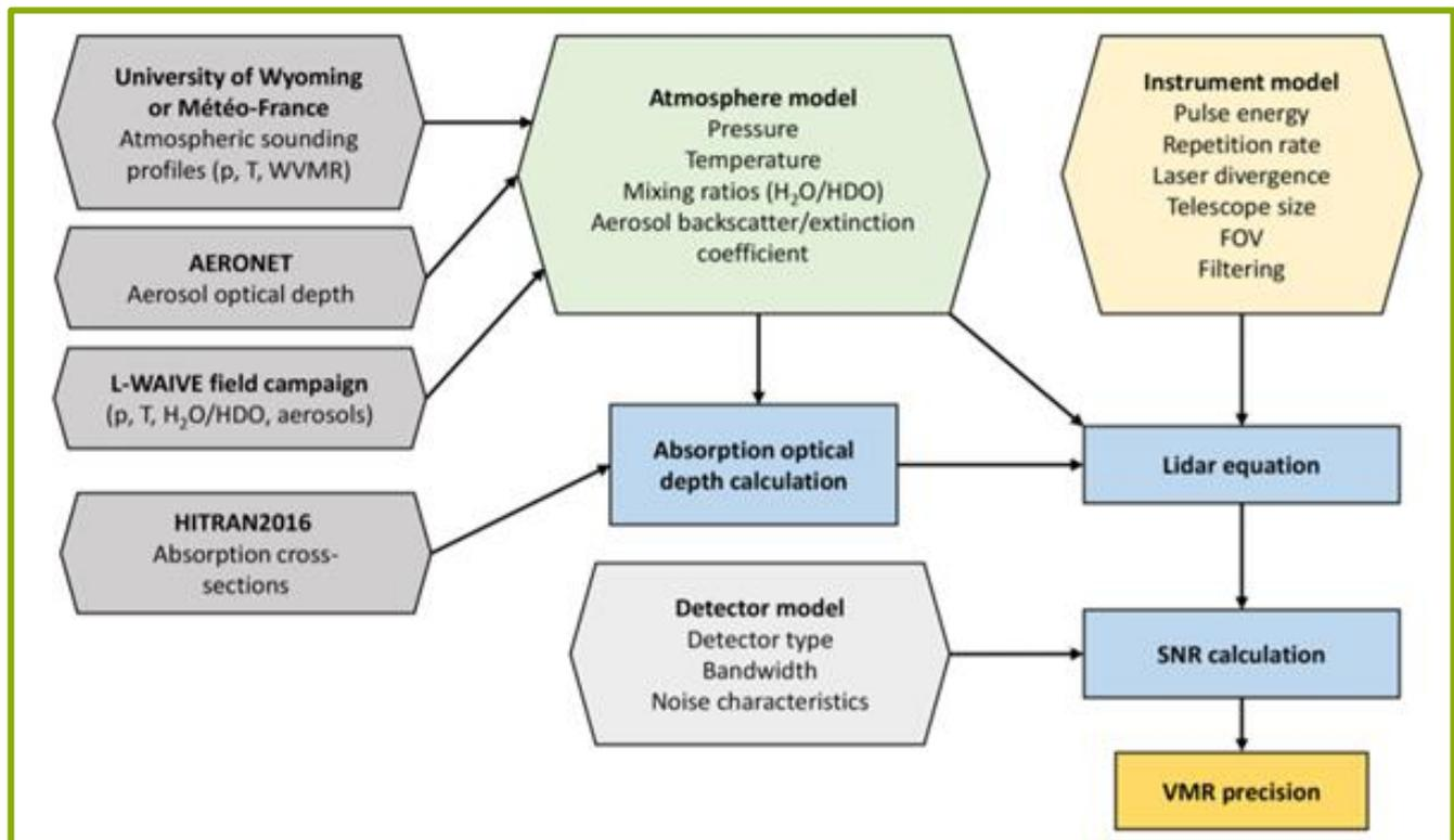
**Figure 7: Block diagram of the DIAL simulator. Input models and databases are in hexagons, and principal calculations are indicated by rectangles. *p*: pressure; *T*: temperature; *WVMR*: water vapor mixing ratio; *FOV*: telescope field of view. The signal-to-noise ratio (*SNR*) is used to calculate the statistical random error (precision) of the volume mixing ratio (*VMR*) of  $H_2O/HDO$ .**
