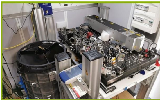
Figure 5: WAVIL DIAL laboratory system consisting of laser bench (right) and reception telescope (left) a). Preliminary WAVIL water vapour volume mixing ratio (VMR in %) and comparison with weather balloon radio-sounding (RS) b). Preliminary HDO volume mixing ratio (VMR in %) and comparison with HDO content calculated as the water vapour weather balloon radio-sounding (RS) and a supposed isotopic ratio \delta D of -100 per mil c). Error and biases sources are to be investigated in the coming weeks.
