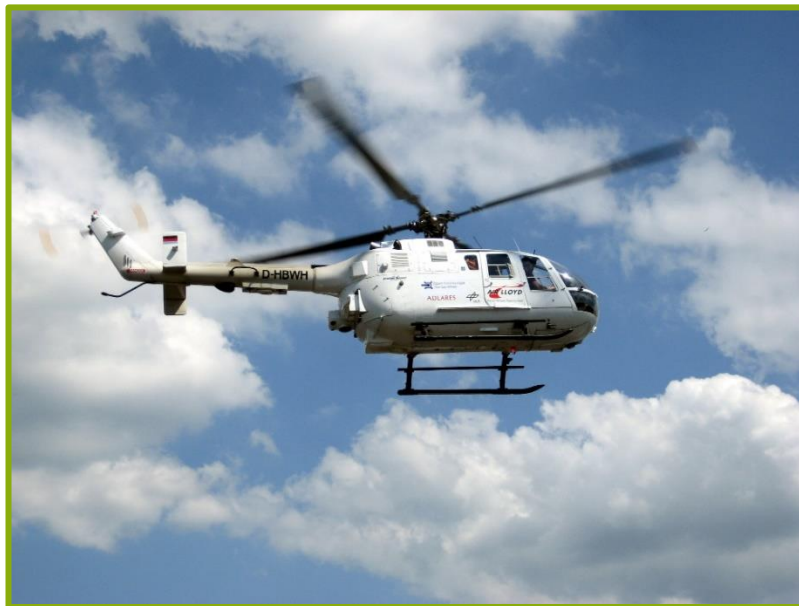
Figure 9: BO 105 helicopter on which Open Grid Europe currently operates the CHARM Lidar System for Pipeline Monitoring.
