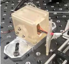
THE LEMON CONCEPT IS BASED ON A GENERIC TUNEABLE FREQUENCY CONVERSION UNIT (GFCU) which converts a  $1\mu\text{m}$  pump laser radiation into two wavelength tuneable radiations to match the targeted species absorption lines.
